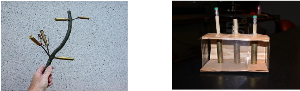
Figure 5: Use available materials to avoid adding your own prints, or smudging the ones already there when you collect and ship the casings
